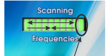
Power indicator LED stays on all the time, while other lights oscillate back and forth.
