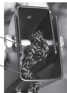
Double knot around bolt
