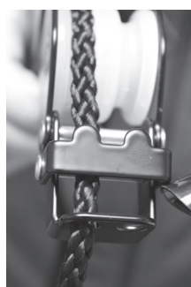
Proper rope placement in brake
