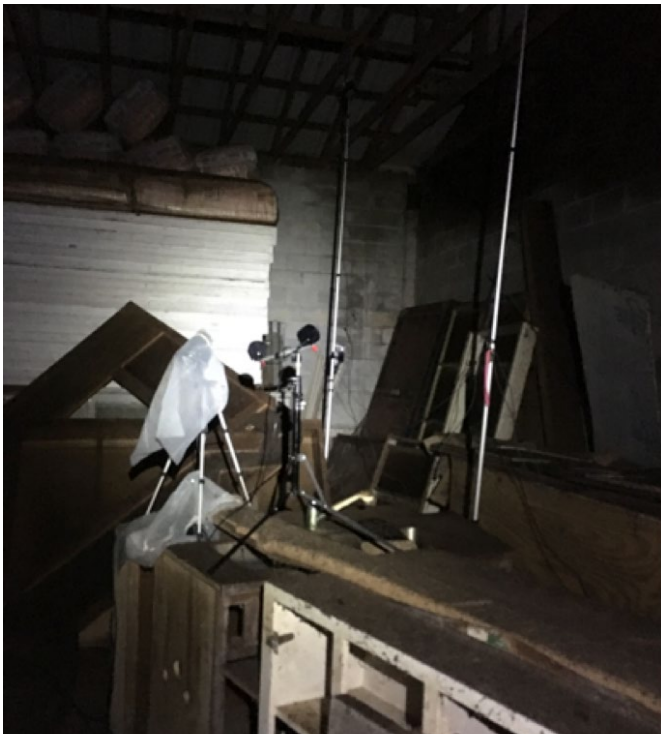
Photo E-4 North end infrared time-lapse camcorder with external infrared lights, ultrasound emitter pole (background), and data logger pole (foreground)
