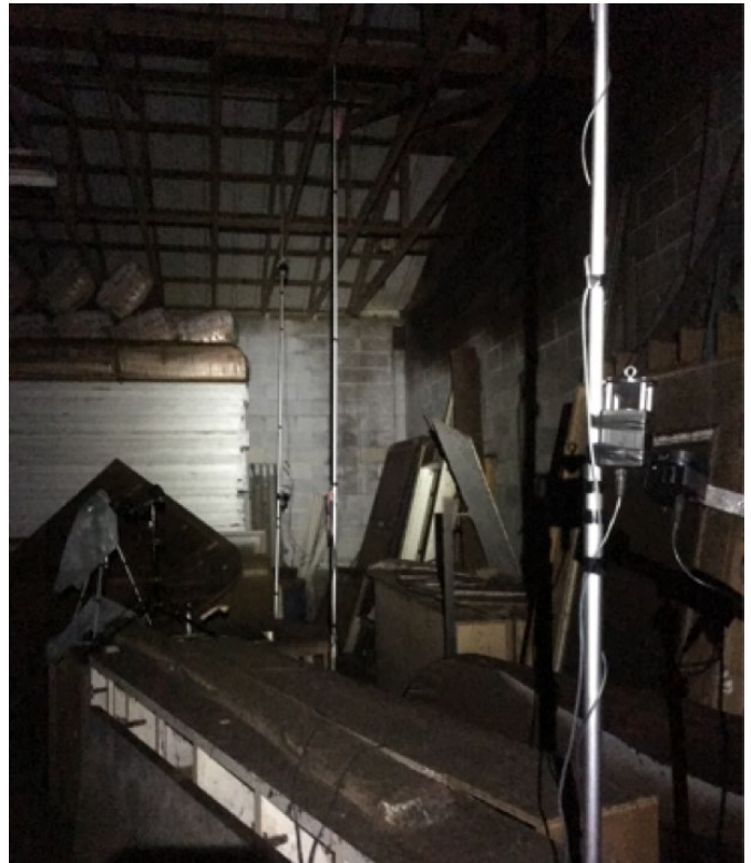
Photo E-5 North end ultrasound emitter pole (background), data logger pole (middle), south end ultrasound emitter pole (foreground)
