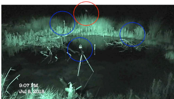
Photo B-11 Site 5 infrared video, treatment data collection; ultrasound emitters circled in blue, bat fly-by circled in red
