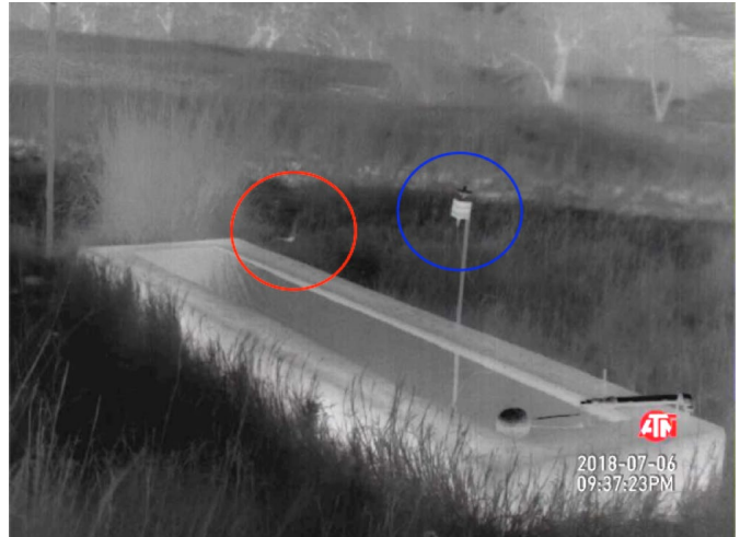
Photo B-8 Site 1 thermal imagery, treatment data collection; ultrasound emitter circled in blue, bat fly-by circled in red; bat appeared to approach water for a sip then turned away
