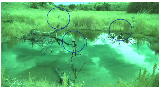
Photo B-12 Site 5 infrared video, treatment data collection; ultrasound emitters circled in blue
