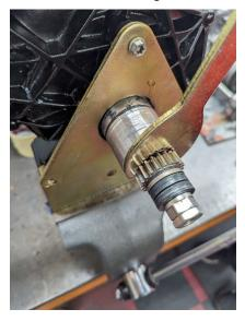
Use an 18mm socket to remove the two nuts on the rear of the shaft.
