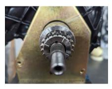
Now take the remaining rollers and slide them into the remaining gaps between the gear and the shaft. You may need to use a pick to move the rollers around under the gear to make room. All 32 rollers should fit under the gear.
