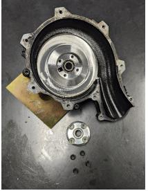
**Step 6)** Press the ball bearing out of the center of the supercharger housing from back to front. When supporting the supercharger in the press make sure that the housing is flat against the supports and not resting on the dowel pins.
