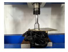
When finished, the bottom plane of the flange on the rear of the supercharger should be approximately flush with the back of the housing, or very slightly below flush.
