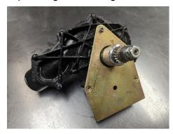
**Step 2)** Use an E8 Torx socket to remove the 9 bolts holding the supercharger housing together.
