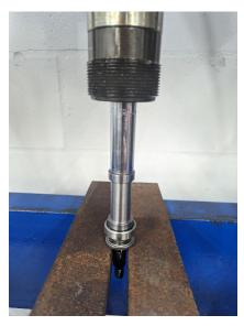
**Step 9)** Install the bearing retainer, making sure to align the circular relief on the back of the bearing retainer with the oil
