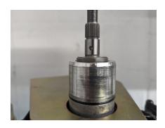
**Step 12)** Install the supercharger impeller wheel.
