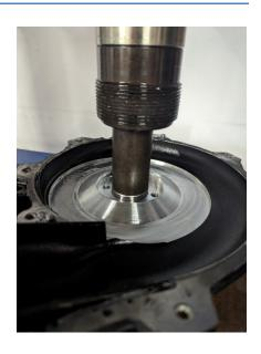
**Step 7)** Press the new ball bearing (part #08) in from the front of the supercharger until it bottoms out. Be careful not to use too much pressure; this bearing should be easy to install.
