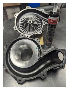
Using an E8 Torx socket, tighten these bolts to 80 inchpounds, in a crisscross pattern.
