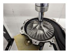
Stop when the bottom surface of the impeller wheel is flush with the inside of the housing.
