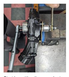
Start by setting the wrench at 130 inch-pounds and try to turn the acorn nut. The wrench should click before the shaft turns. If the shaft turns without the wrench clicking first, tighten the rear nut a little more (as in step 17) and check the slip again. Continue this process until the wrench clicks at 130 inch-pounds without turning the shaft. Then change the torque setting to 145 inch-pounds and attempt to turn the acorn nut.
