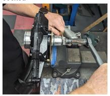
The supercharger is now rebuilt. You can follow this process to check the slip again after the supercharger has been used to determine if it needs to be rebuilt; a good used supercharger should slip at 100 inch-pounds or more. Less than 100 inch-pounds indicates that the supercharger should be rebuilt. SBT recommends that you check the slip on the supercharger after 100 hours of use.
