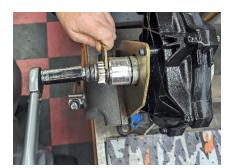
**Step 18)** Set the slip torque of the supercharger. A new 300 supercharger should slip at 125 to 150 inch-pounds.
