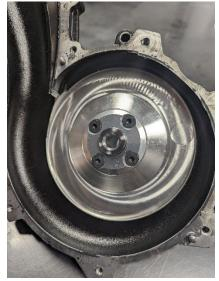
installation. Support the center shaft by the flange; do not stand it on end.
