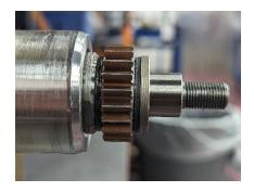
Lubricate with motor oil and slide the 8 cupped spring washers (part #12) over the spacer in this order:
