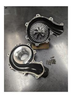
**Step 3)** Disassemble the clutch on the back of the supercharger.
