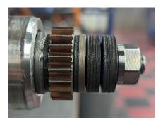
Step 17) Hold the flange of the supercharger shaft with the special wrench (SBT part #80-300-01) and tighten the nut on the back of the supercharger shaft to approximately 20 footpounds using a torque wrench and an 18mm socket. The exact torque of this is not critical because we will adjust it based on the slip of the clutch in the next step.
