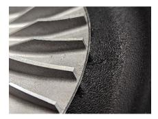
Check that the impeller wheel spins freely and does not rub the housing. If the impeller wheel rubs, repeat step 4 to disassemble and repeat steps 11 and 12 to reinstall.
