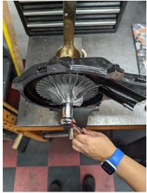
Support the supercharger securely in a press and push the shaft towards the back of the supercharger to release it from the impeller fan wheel. Push until the end of the shaft is flush with the fan wheel to release it; there is no need to push it through the fan wheel. Take care not to press on the
