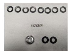
Slide one of the flat friction washers over the end of the shaft until it touches the flange. Apply a liberal amount of grease to the shaft to help stick the rollers to shaft. Peel the rollers off the tape they are stuck to, making sure that no adhesive remains on the rollers, and stick them to the grease on the shaft. Add more grease as needed to keep the rollers on the shaft. Stop when you have at least 6 rollers left.
