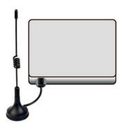
iPETRO Tank comes with a passive internal GSM antenna (SMA connector) on CON6. However, if the device is mounted inside a metal enclosure, it might be hard to obtain good reception. In such cases, connect an external GSM antenna, run the cable through one of the glands at the bottom of the casing, and make sure the antenna itself is located as high as possible to ensure good mobile reception.
