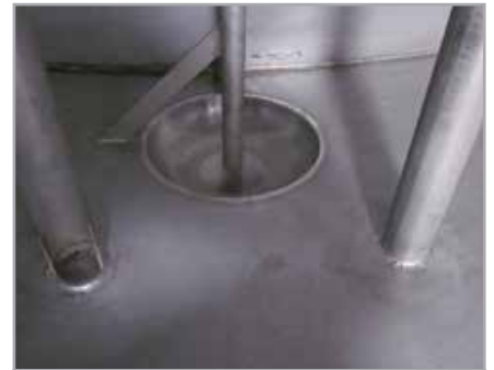
Water Sump & Extraction Point
