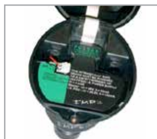
Inside of I.S. IMP (ATEX and IECEx)
