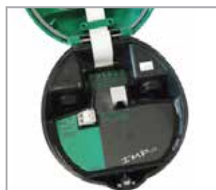
Inside of IMP Lite showing RJ11 Port
