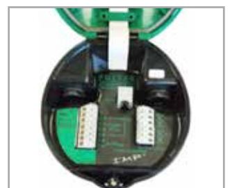
Inside of Standard 2/3 wire IMP
