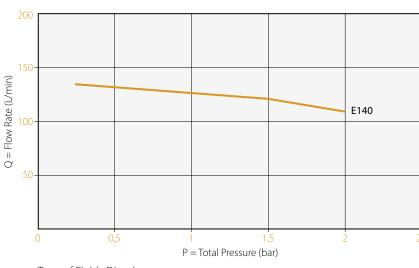
Type of Fluid: Diesel Temperature: 20 °C
