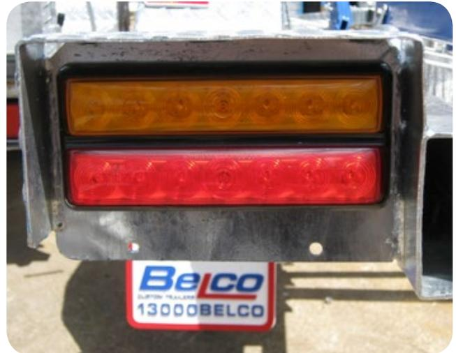
**NEVER** use hazard lights to check indicator function, as they may not show faults. Each light should be checked individually.
