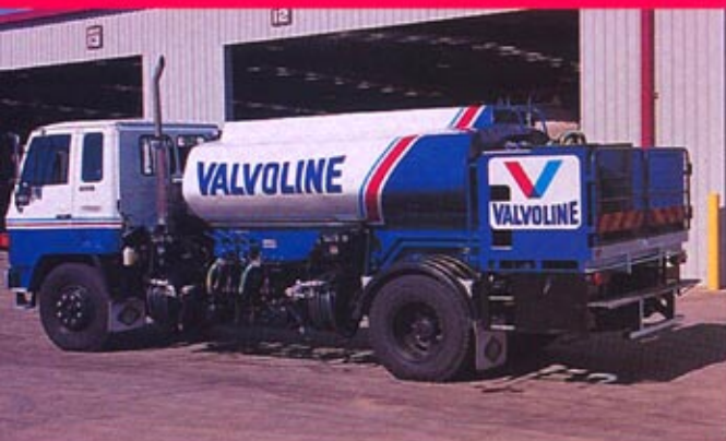
Tanker Mounted Pumps
