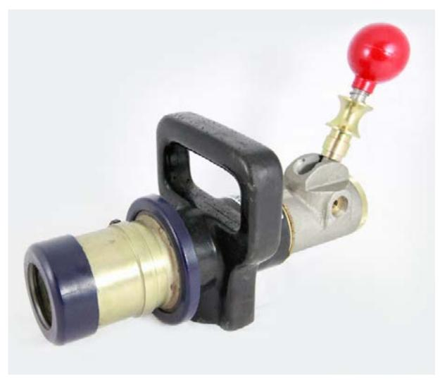
Specifically-designed for underground refuelling of diesel-powered machines, the Underground Nozzle is Dry Break, offers improved dispensing rates, and is manufactured without aluminium, for use in coal mines.
