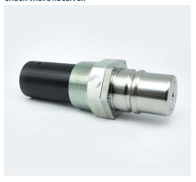
Our Check Valve Receiver integrates fuel security along with Dry Break functionality. It prevents unwanted fuel drainage from the tank which stops theft, and allows for the receiver front-end to be replaced without having to drain the tank first. This saves time on scheduled maintenance, and money because only the worn part is replaced.
