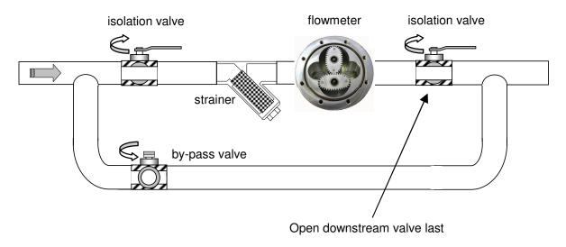
After flushing or following long periods of shutdown the meter must be purged of air/vapour. This can be achieved by allowing the liquid to flow through the meter at a slow rate until all air/vapour is displaced. Never run the meter above i ts maxi mum How or exceed 100kpa (1 bar. 15psi) pressure drop across the meter. Now the meter is ready for its operation to be confirmed by ensuring correct indication on the mechanical display. Refer if necessary to fault finding section of this manual.
