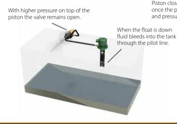
Piston close under spring force once the pilot line fluid bleed stops and pressure is equalised. Float rises with the fluid level, shutting off the bleed through the pilot line.
