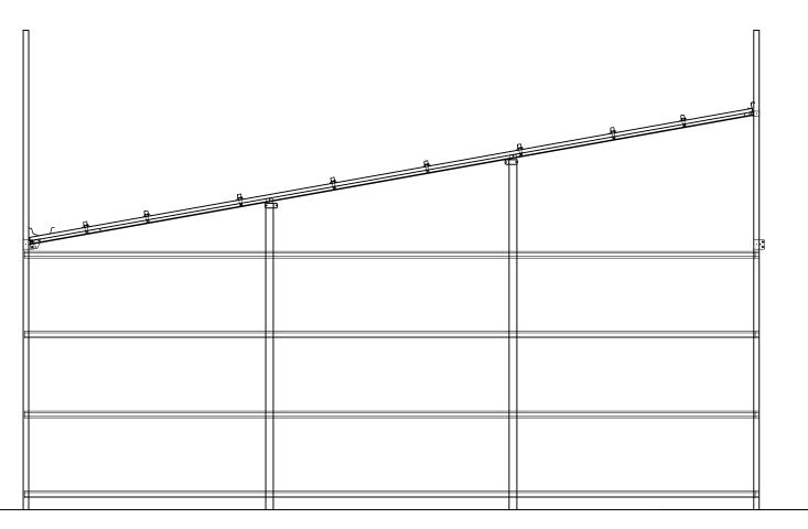
NOTE: ENDWALL COLUMN SPACING ILLUSTRATED MAY VERY TO ACCOMMODATE DOOR SIZING.
