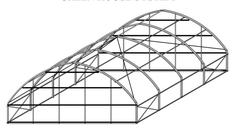
NOTE: ENDWALL COLUMN SPACING ILLUSTRATED MAY VARY TO ACCOMMODATE DOOR SIZING.
