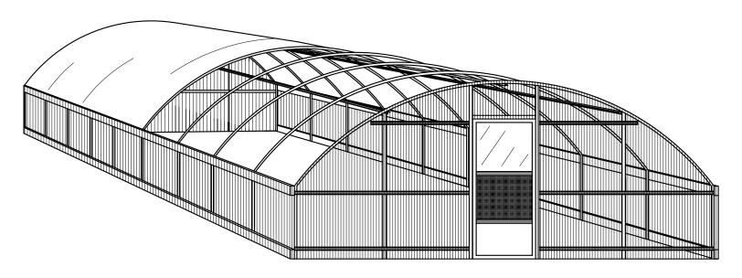
NOTE: ENDWALL COLUMN SPACING ILLUSTRATED MAY VARY TO ACCOMMODATE DOOR SIZING.
