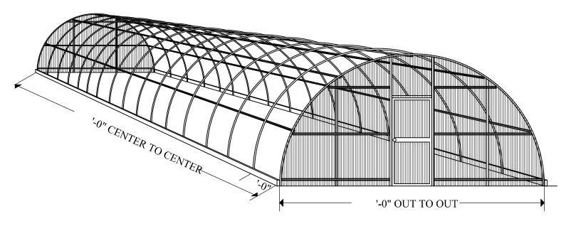
NOTE: ENDWALL COLUMN SPACING ILLUSTRATED MAY VARY TO ACCOMMODATE DOOR SIZING.
