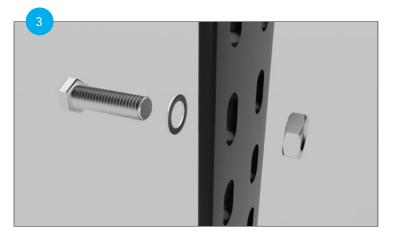
Attach using (x2) Long Bolts, (x2) Washers, and (x2) Nuts. Repeat this step for all sides as needed.
