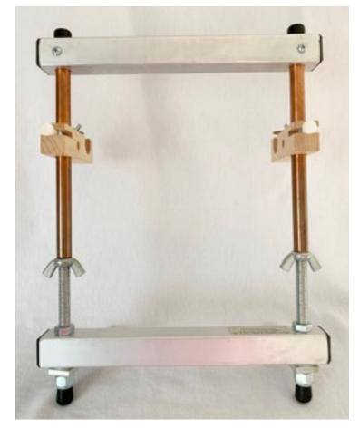
Make sure you have at least an inch of threaded rod exposed at the bottom in order to be able to adjust your loom for rotating the warp to the back. You can extend your loom to the point where the copper covers at least 4" of the threaded rod when warping on the 8, 12 & 16" looms and 6" on the 22, 28, 32 & 38" looms. Going beyond that point will potentially make your loom unstable. Make sure the loom is even on both sides.
