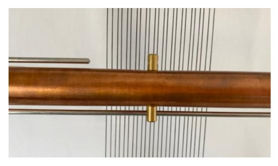
Place heddle around the first warp and loop onto heddle bar. Continue doing this with every other warp. (After this you will put heddles on the other warps and attach those to the other heddle bar allowing each set of warps to be raised separately).
