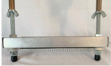
The teeth will stick up from the top beam and down from the bottom beam. We have made the combs loose enough so that they are easily removable and do not damage the aluminum. If your combs are not staying in place tie a string around the comb to hold it in place temporarily. Once you begin warping the combs will stay in place. Remove this as you warp.
