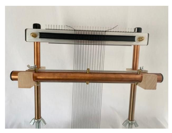
Loosen screw that holds in top heddle bar (the heddle bars are the two bars on the top and bottom of the shedding device that will eventually hold the heddles to create different sheds).
