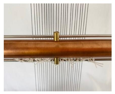
Release screw and reinsert bar. Tighten screws. Make sure bar is flush with the side of the stand-off that the bar goes through.
