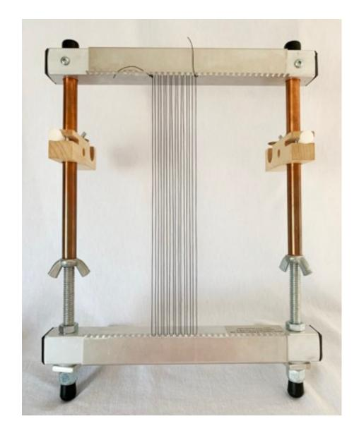
When you have warped as far across as desired, tie off on any tine and then tighten your tension by turning your loom's wing-nuts counter-clockwise.
