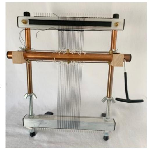
Above the bottom beam, where you want your weaving to begin weave in a length of warp, wrap around the copper side bar, weave back to beginning and tie the two ends around the other copper side bar. You can start your piece anywhere on the loom, but may want to start higher up to ensure you have enough warp waste for finishing.
