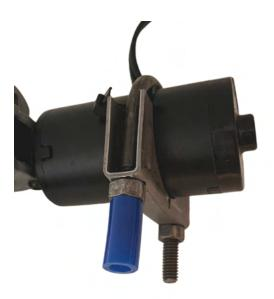
Blue or Yellow Bushing (installed on motor)
