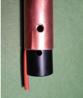
The motor shaft is inserted into the bushing but needs to be aligned with the hole in the bushing as well as with the frame of the loom. The motor is assembled so as to fit most looms but fine adjustment might be necessary. On some looms, it may be necessary to loosen the U-bolt before the motor will fit at all.
