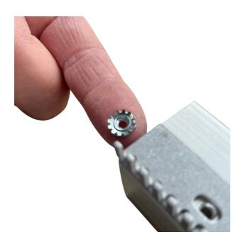
To replace the combs, line up the holes in the comb to the holes on the beam. Make sure that the tines are on the edge of the beam. Slide the nut inside the square tube on your finger tip until you can see it is lined up with the hole. Screw in the bolt while holding the nut until snug. Helpful tip, wrap a piece of tape, sticky side up, on your finger to hold the nut.
