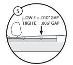
STEP 5. Restring the high and low E strings and tune to pitch to check for correct height. Pushing down on the third note of the low E string should result in a .010° gap between the string and the first fret; high E string should be .006°
