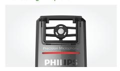
The free-floating microphone is decoupled from the device's housing, which guarantees that almost no background, touch, click, air or structure-borne noise is recorded.
