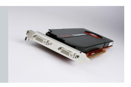
The MXRT-5450 is a high-performance PCIe display controller featuring AMD FirePro  $^{\mathsf{TM}}$  3D technology for leading-edge performance, flexibility and reliability. The board supports DirectX and OpenGL and is compatible with Microsoft Windows® XP and Windows® 7.
