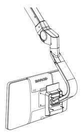
3. Plug the power cable in the power connector of the display panel. Attach the other side of the cable to the power cable of the VESA arm.
