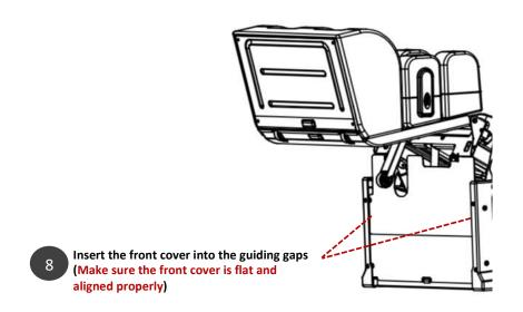
Fig.6: Footrest Assembly: Chair Front Cover Reset
