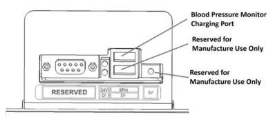
Fig.9: Blood Pressure Monitor Charging USB Port
