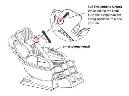
Fig.21: Bicep/Shoulder Massager Position Adjustment
