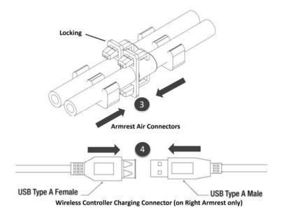
Fig.8: Armrest Air and Electrical Connections
