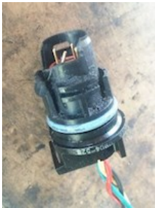
Damaged Ford 6.0 Injector Plug
