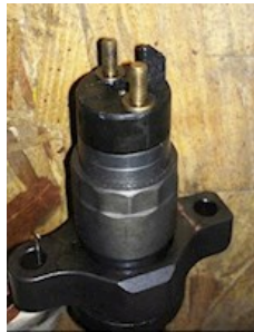
Damaged Dodge CR Injector
