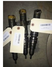
Damaged CAT C7/C9 Injector
