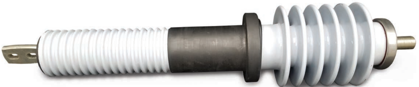
34.5kv, 200kv BIL, 1200 Amp, air-air switchgear bushing.
