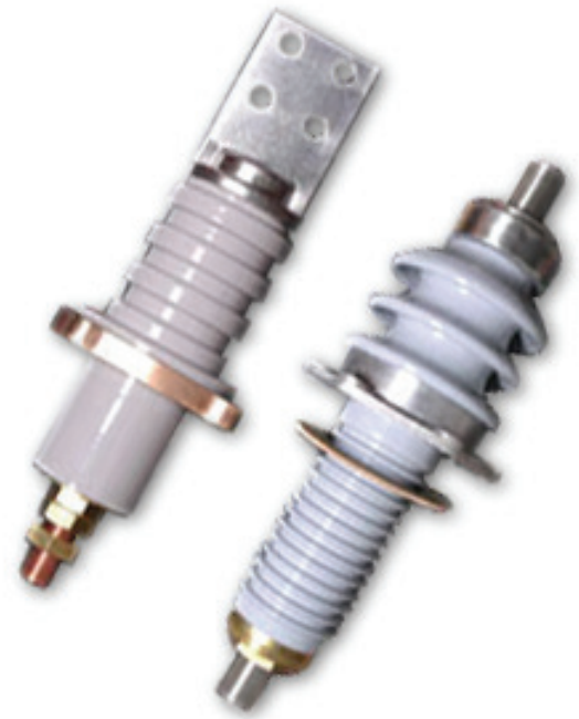
34.5kv, 200kv BIL, 1200 Amp, air-air switchgear bushing.
