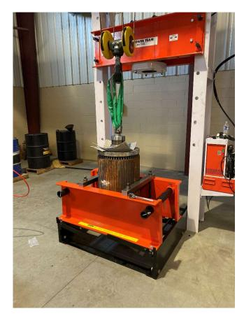
Once armature is in fixture, remove lifting device.
