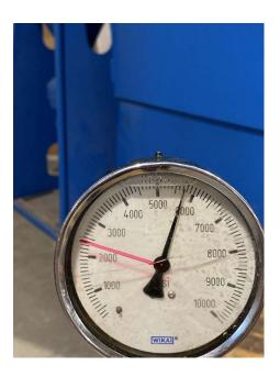
• Final gauge reading on hydraulic pump should be around 5800 PSI.
