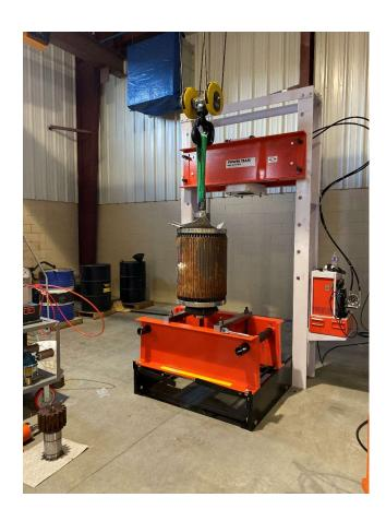
Load armature in center of fixture
