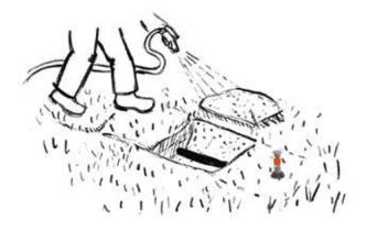
Now pour the soil back in, put the turf on top and tread it down. If you water the soil and the turf first, everything will grow faster. And in 2 to 3 weeks you won't see any more of the installation.
