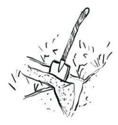
Use a spade to dig v-shaped trenches approx. 20-25 cm deep. To do this, carefully remove the trenched and dig out the trench. Remove the stones from the trench. Tip: Mow the lawn and water it beforehand. Then it's easier.
