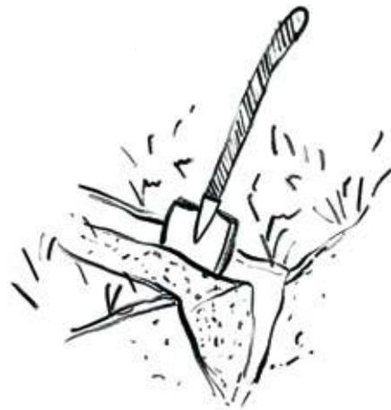
**F** Use a spade to dig v-shaped trenches approx. 20-25 cm deep. To do this, carefully remove the trenched and dig out the trench. Remove the stones from the trench.
