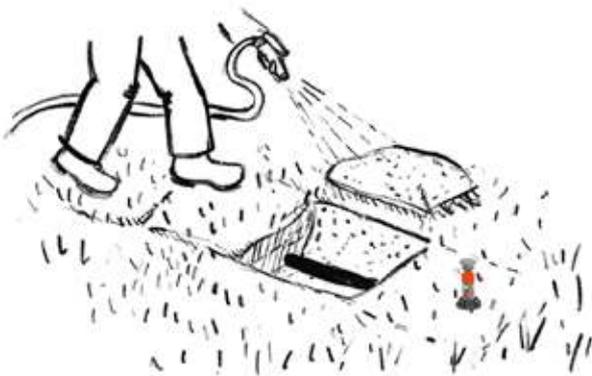
**I** Now pour the soil back in, put the turf on top and tread it down. If you water the soil and the turf first, everything will grow faster. And in 2 to 3 weeks you won't see any more of the installation.
