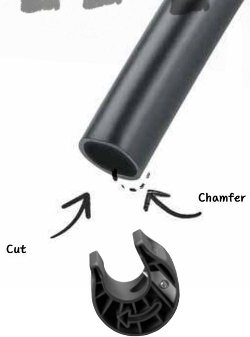
**B** Cut the Pipes to the right length according to the plan. Make sure that no soil gets into the pipe. If necessary, chamfer the pipe, i.e. remove unclean cut edges. For straight Pipe cuts in just one turn, use the GARDENA Pipe Cutter for cutting the Connecting Pipes (Art. No. 2727).
