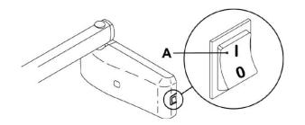
The control unit is turned on and off from the main switch (A).
