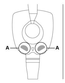
In the versions equipped with ball joint, the x-ray head can freely rotate on both its horizontal and vertical axis.
