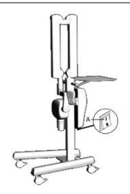
The control unit is turned on and off from the main switch (A).
