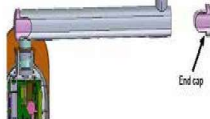
Figure 34 Fix end cap (M3x6 self tapping Counter sunk screws )Use screw driver
