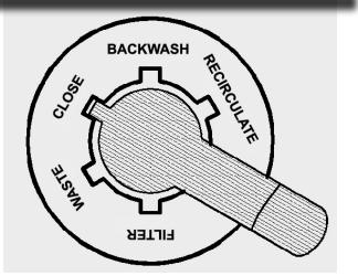
1.Filter - Position for filtering the body of water.
