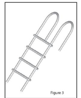
Slide the second hand rail through the hole on the opposite side of the step. Secure with a nut and bolt.
