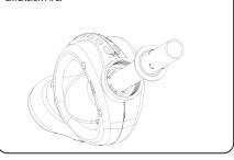
(h) Screw the HANDNUT into place to lock the assembly. **Be careful not to over-tighten the Handnut.**(i) Check that the OUTER EXTENSION PIPE swivels freely.
