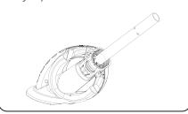
(f) Slide the THRUST WASHER over the INNER EXTENSION PIPE. The flat side (widest diameter) of the THRUST WASHER should face down.
