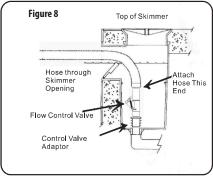
The Flow Control Valve is preset between positions 3-4. This provides the ideal operating flow in most pools. If necessary, the flow can be adjusted by using any setting from position 1 through position 6 (1= min flow, to slow your cleaner down, 6= max flow, your cleaner will run faster). See Fig 9.
