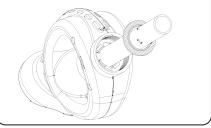
(g) Place the OUTER EXTENSION PIPE over the INNER EXTENSION PIPE.
