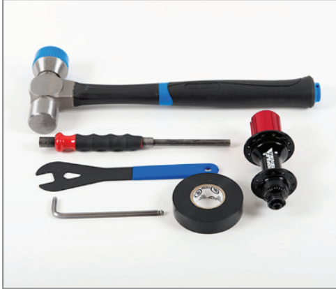
Tools Required: Hammer, punch or bearing press, 17mm cone wrench, 5mm allen wrench and bearing removal base
