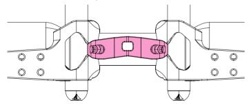
Install the bridge piece into the supersonic brackets using the 4mm hex wrench, and use the 4mm torque fitting to tighten the mounting bolts to 4Nm.
