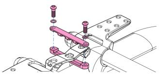
\*Make sure the mounting plate is sitting securely in the square hole on the bridge before tightening the cage mounting bolts to 3Nm.
