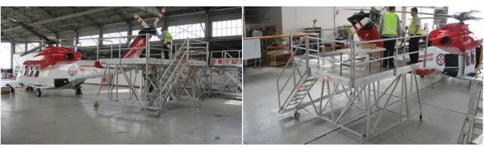
Ensure safe, easy and hassle free access for maintenance on helicopter tail rotor
