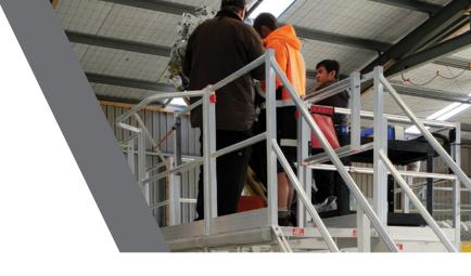
Like many of SafeSmart's platforms, this system for HNZ Group is easily wheeled by hand up to the aircraft and secured into place via foot-lockable castors.
