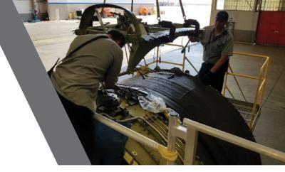
United's technicians can wheel two of SafeSmart's identically-mirrored arched access systems together to form one safe bridge over the aircraft's engines.
