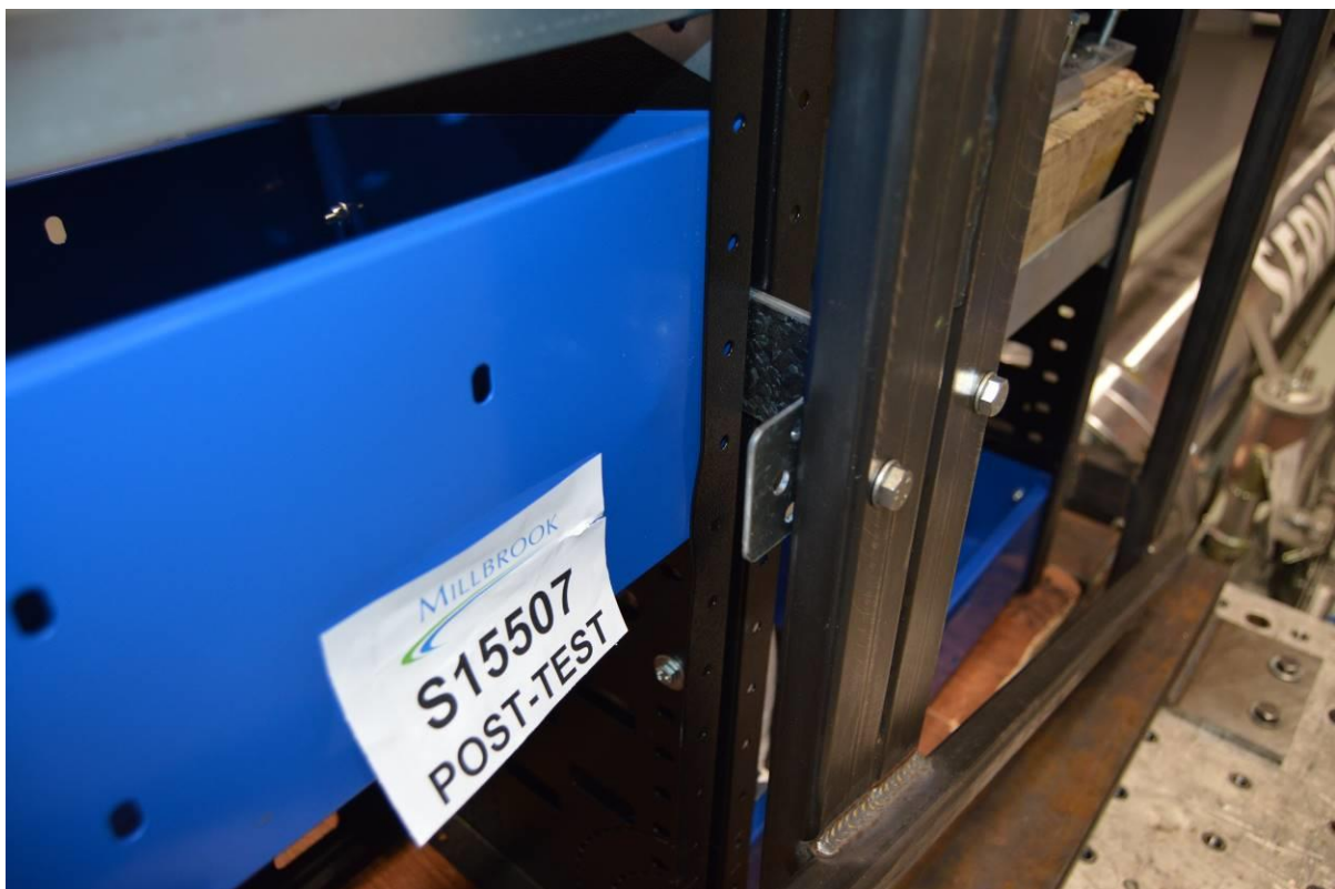
Close-up of Extra-Heavy-Duty racking lower mount, post-test
