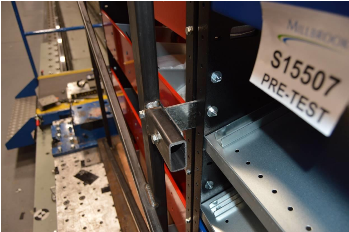
Close-up of StoreTidy/Standard-Heavy-Duty racking upper mount, pre-test
