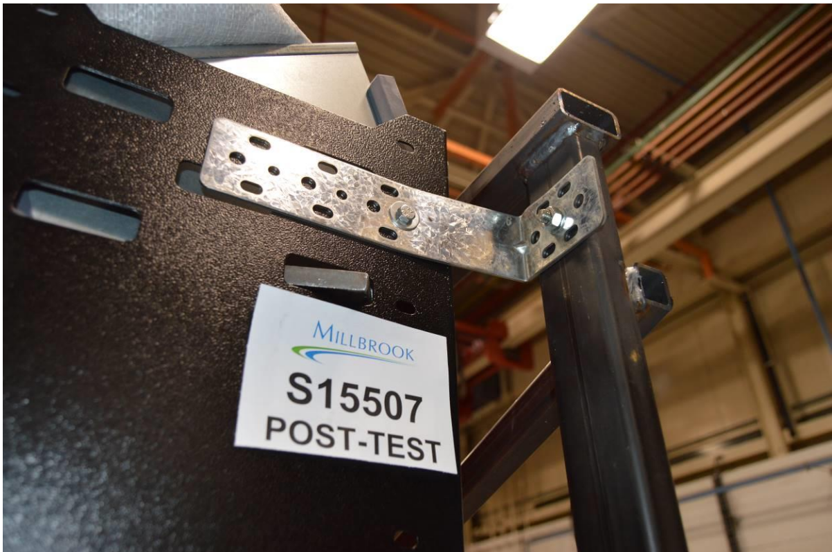
Close-up of StoreTidy racking upper mount, post-test
