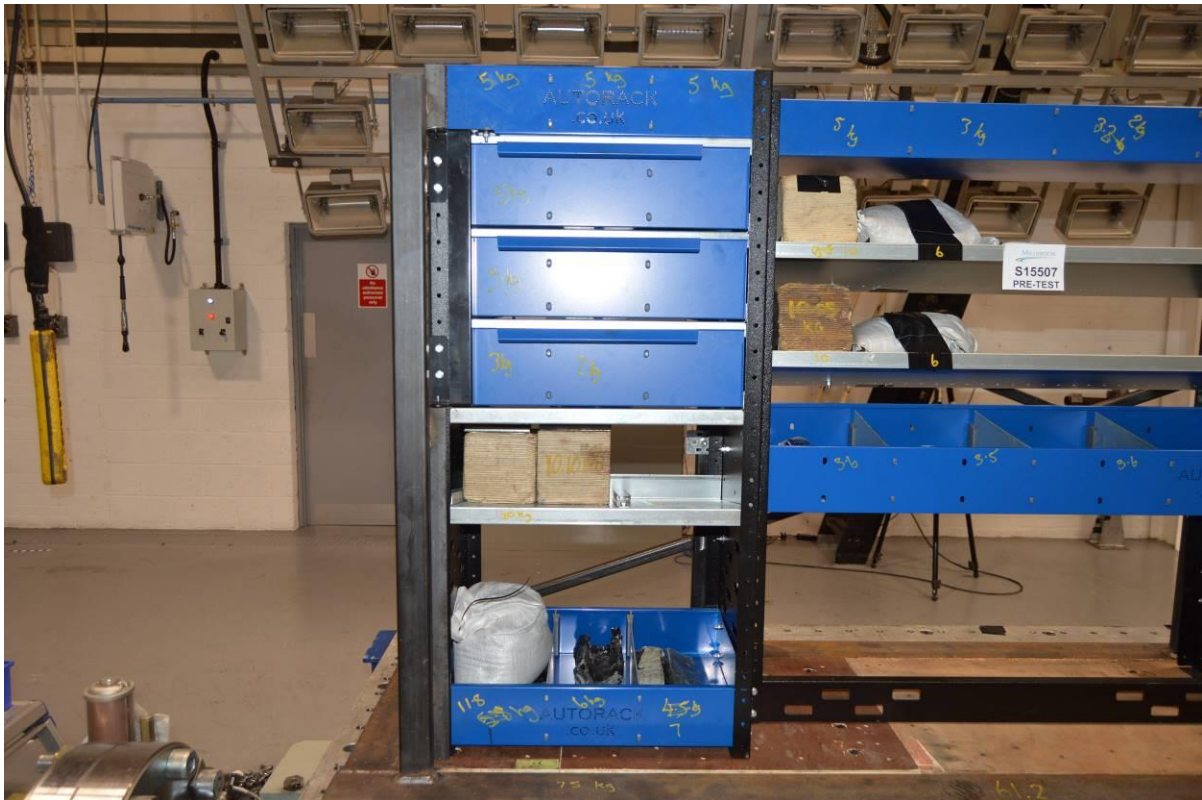
LH close up of Extra-Heavy-Duty van racking, pre-test
