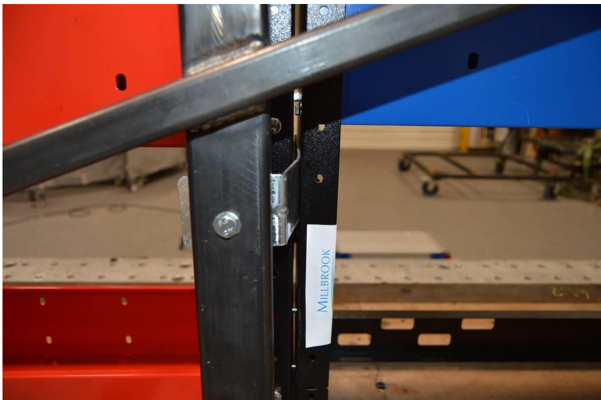
Close-up of StoreTidy/Standard-Heavy Duty Racking mounting bracket, post-test
