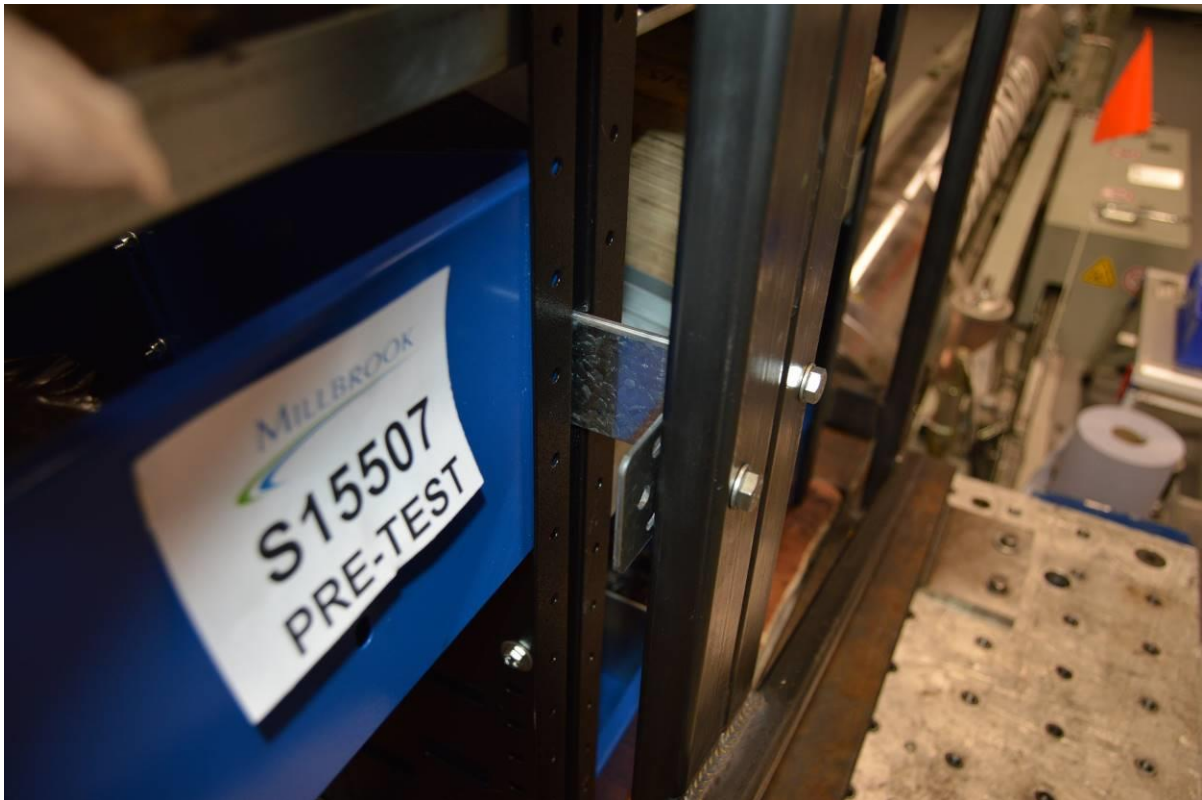
Close-up of Standard-Heavy-Duty/Extra-Heavy-Duty racking lower mount, pre-test
