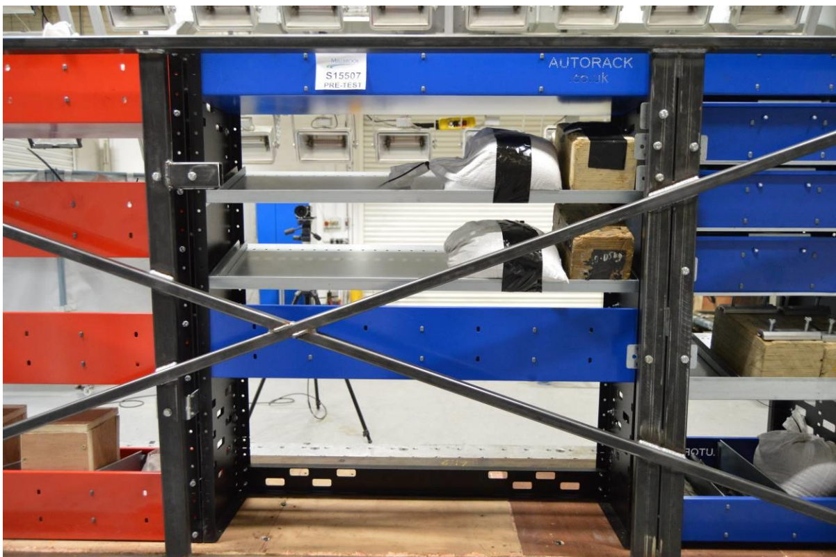
RH close up of Standard-Heavy-Duty van racking, pre-test
