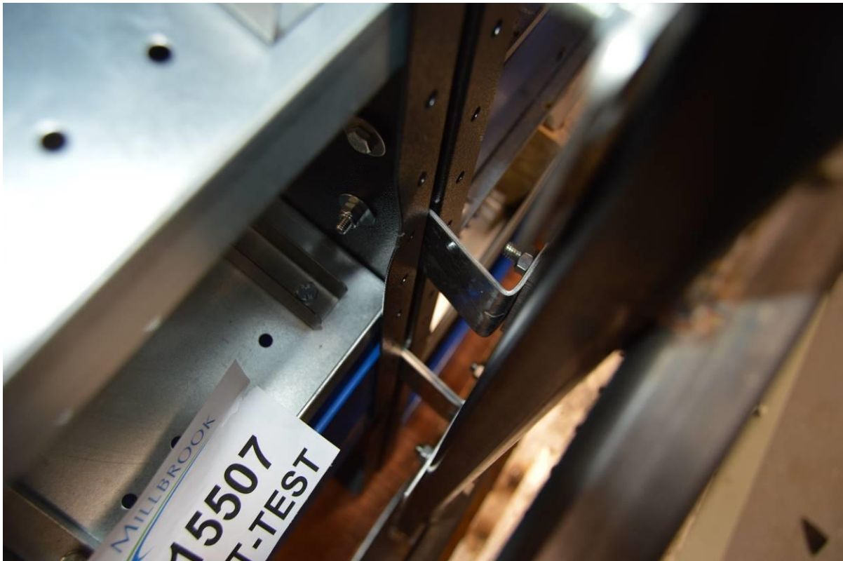
Close-up of Standard-Heavy-Duty/Extra-Heavy-Duty racking, post-test
