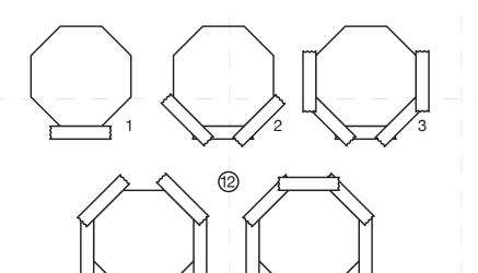
12. Tape over moisture barrier cut lines and exposed nails with flashing tape. \* for brickmould, tape along with a 3/4" overlap on brickmould.
