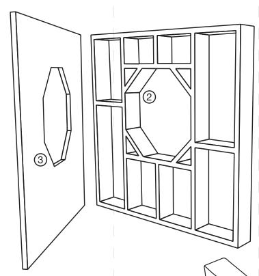
2. Build rough opening and install corner braces per recommended inside measurements (see 1). 3. Trace rough opening and cut out
