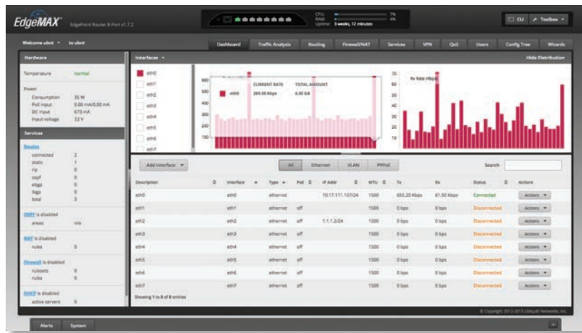
For the EP-R8, the Dashboard screen displays detailed statistics: IP information, MTU, transmit and receive speeds, and status for each interface.
