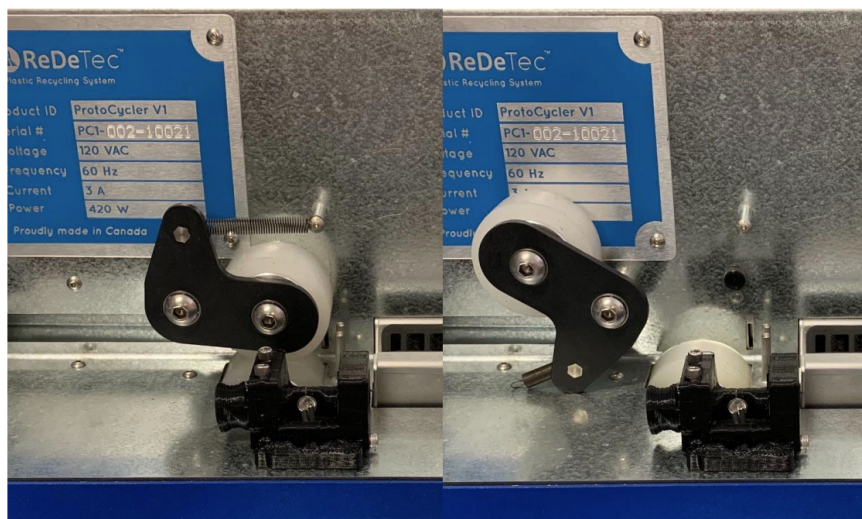
Figure 5: Puller idler wheel spring engaged (left image), and disengaged (right image).
