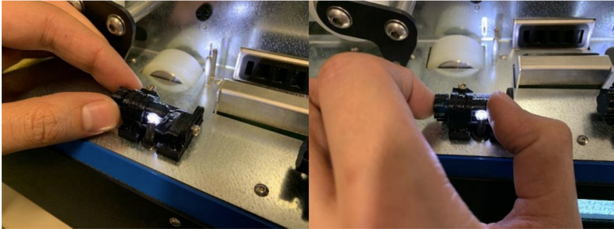
Figure 12: How to grip the light guide shaft to adjust LED angle.
