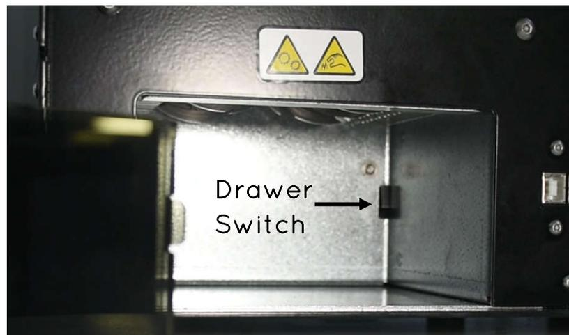
**Figure 3.8 Grinder Drawer Interlock Switch**
