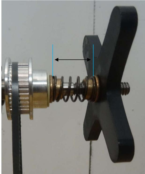
**Figure 3.7 Spooler Clutch Spring Length**
