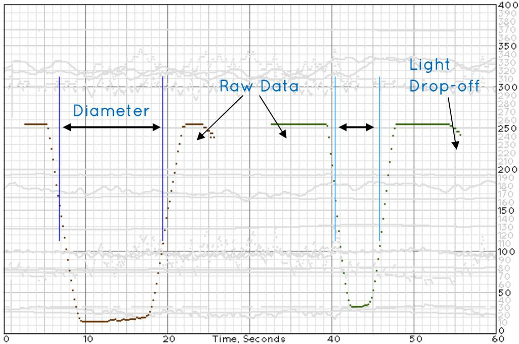
**Figure 3.3 Ideal Sensor Reading**
