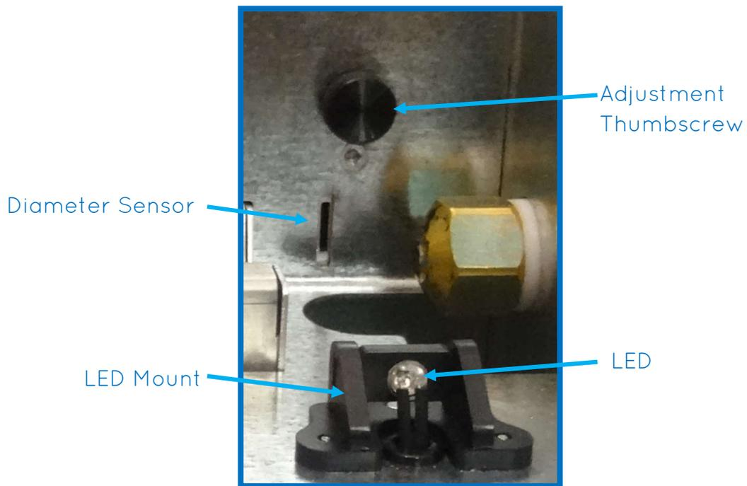
**Figure 3.1 Filament Sensor Close-up**
