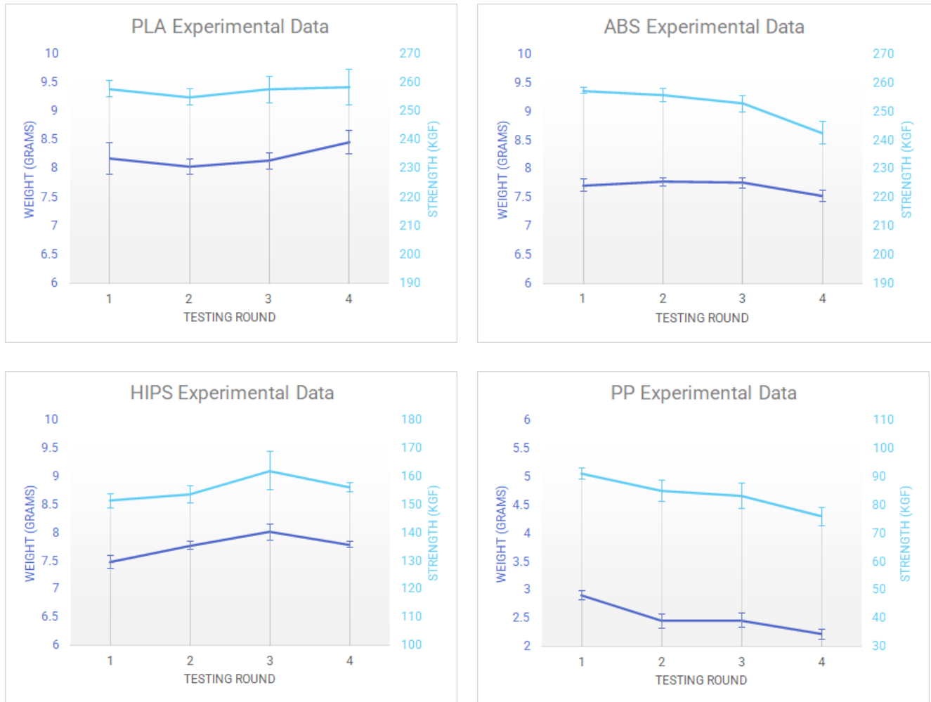
Figure 3.2: Weight and Max. Tensile Strength Averages for each round. Error bars represent +/- 1 SD. (axis ranges are equally sized with a 4g weight range and a 80kgF strength range, and have been offset to center the data).
