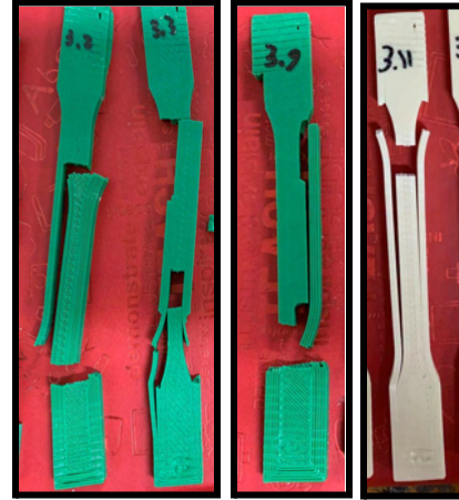
Figure 3.3.2: Examples of undesired failure. ("messy" fracture(s) parallel to the loading axis and outside tapered region of dogbone).
