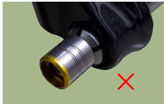
Figure 9. Improperly Secured Axle - Not Expanded
