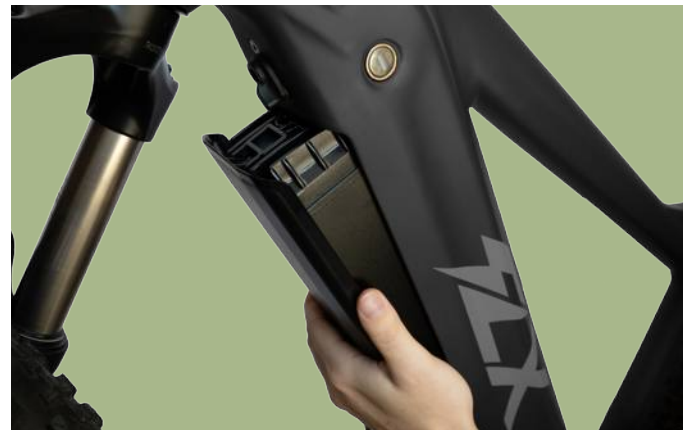
Figure 16. Removing the Battery
