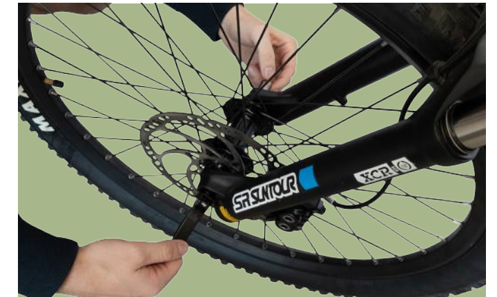
Figure 7. Tightening the Thru Axle
