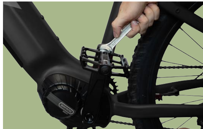
Figure 12. Attaching Pedal to Crank
