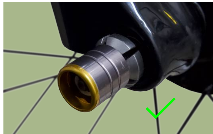
Figure 8. Properly Secured Axle - Expanded Fully
