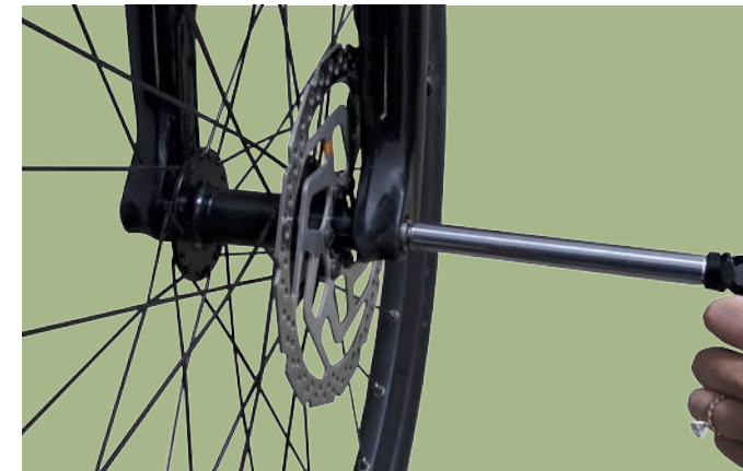
Figure 6. Inserting the Thru Axle
