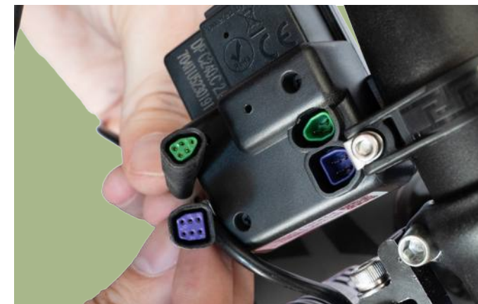
Figure 3. Connecting the LCD cables
