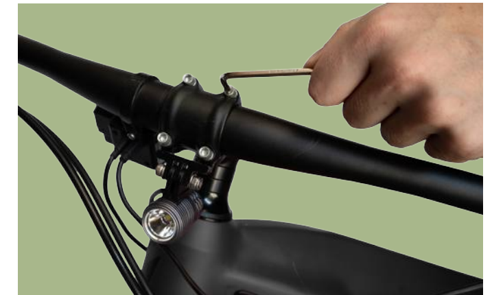
Figure 2. Tightening Stem Plate Bolts
