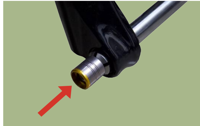
Figure 4. Push to remove Thru-Axle
