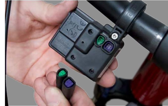
Figure 11. Connecting your LCD Cables
