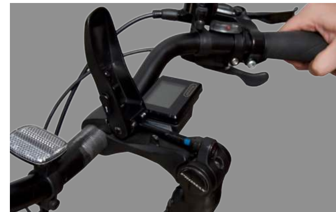
Figure 8. Angling the Handlebars
