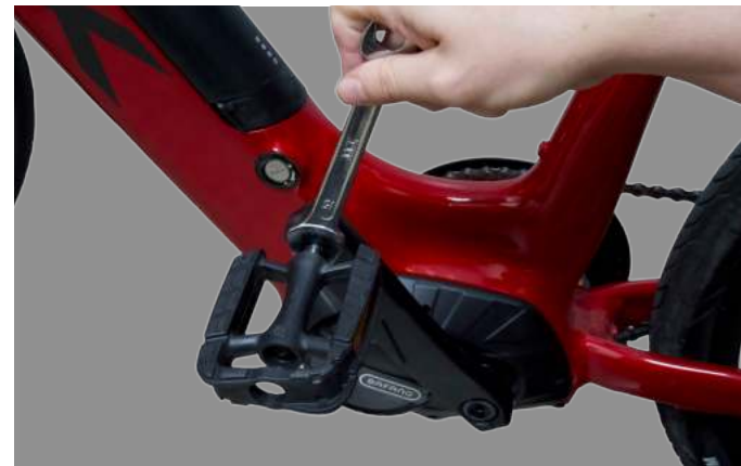
Figure 14. Attaching Pedal to Crank
