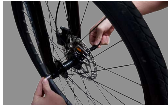
Figure 4. Tightening the Thru Axle
