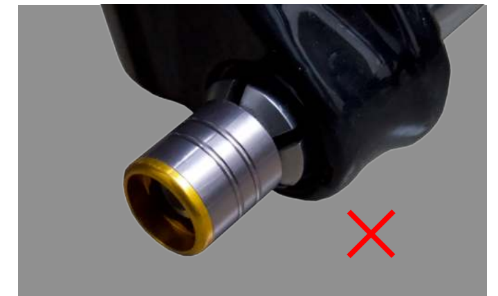
Figure 6. Improperly Secured Axle - Not Expanded
