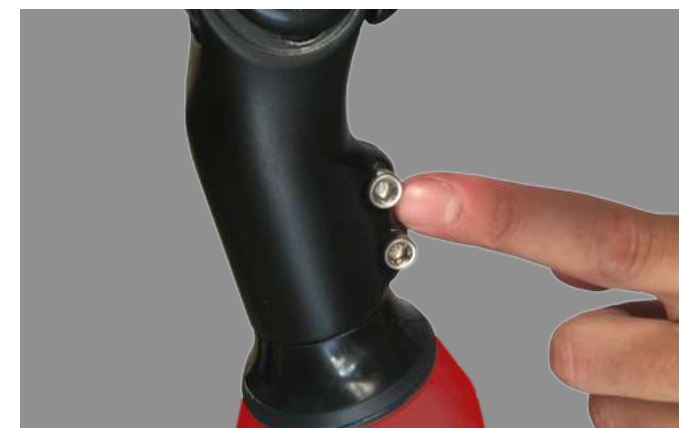
Figure 9. Tightening the Stem Bolts (x2)
