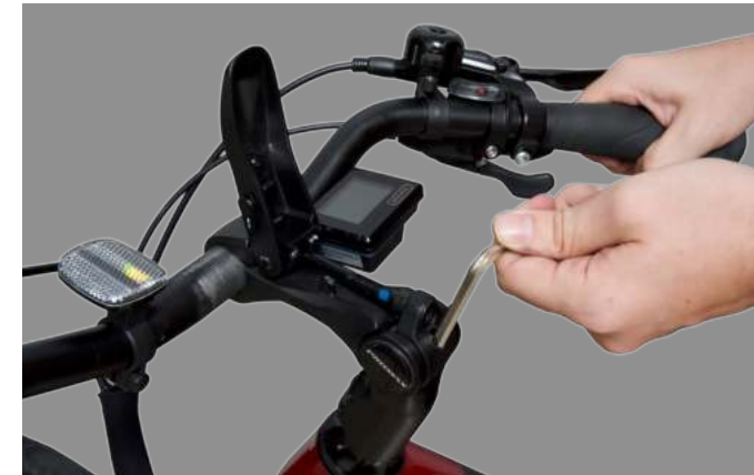
Figure 7. Tightening the Stem Bolt
