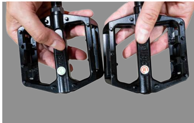
Figure 13. Left Vs. Right Pedal
