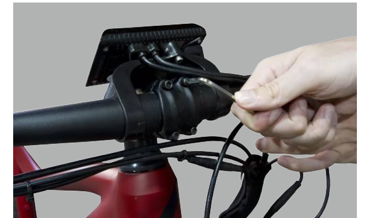
Figure 2. Tightening Stem Plate Bolts
