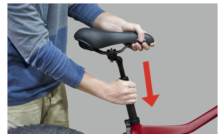
Figure 8. Dropping Seat into Bike
