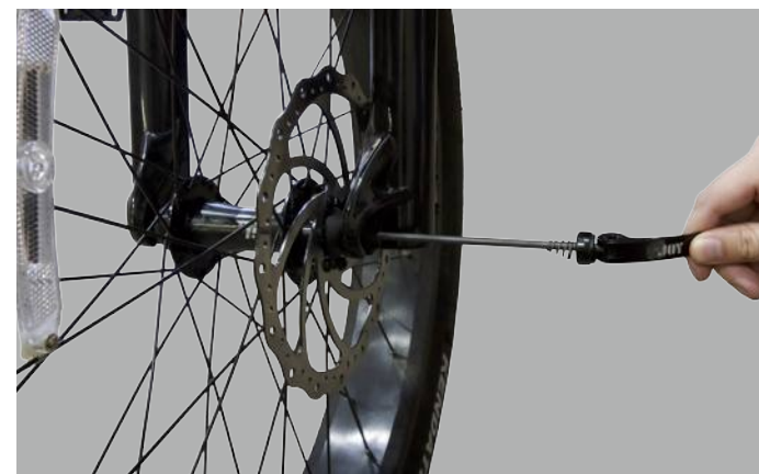
Figure 6. Inserting the Thru Axle
