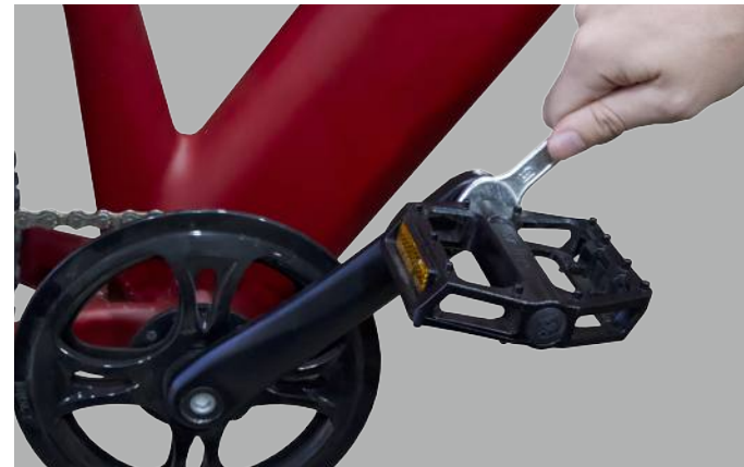
Figure 10. Attaching Pedal to Crank
