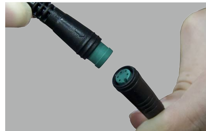
Figure 3. Connecting the LCD cables
