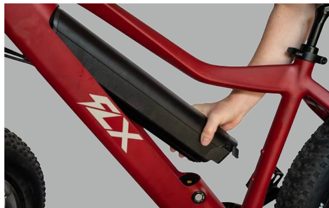
Figure 11. Removing the Battery
