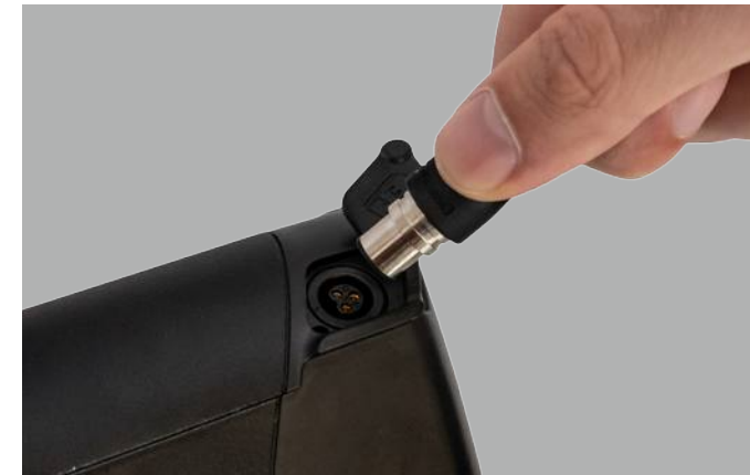
Figure 12. Charging Your Battery
