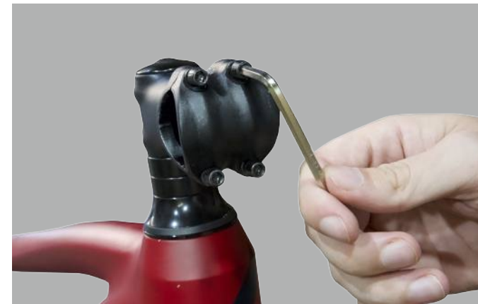
Figure 1. Stem Plate Bolt Removal
