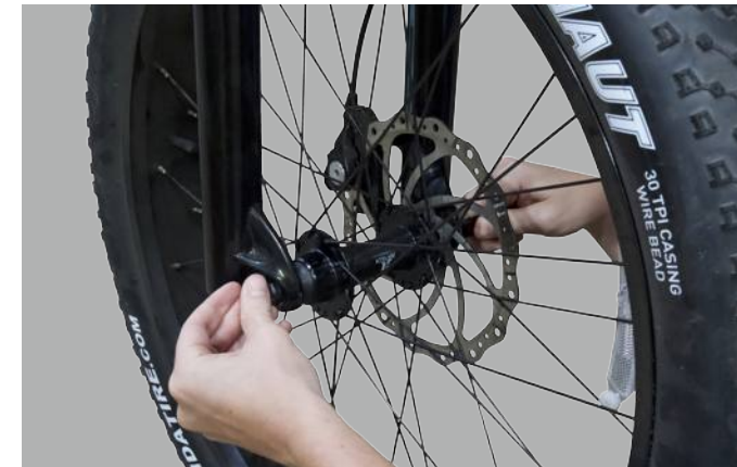
Figure 7. Tightening the Thru Axle
