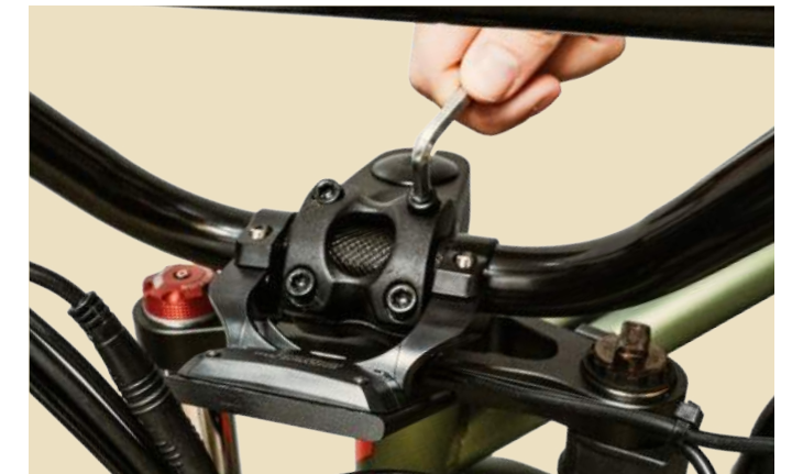
Figure 3. Tightening Stem Plate Bolts
